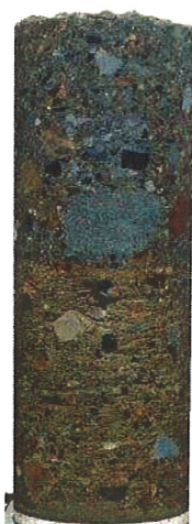
SAMPLED BY GP-R (300mm) FILL MATERIAL OF A ROAD
